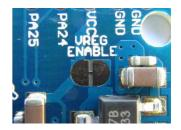
The TS1117-3V3 has a typical dropout voltage of 1,3V @ 1A, maximum 1,5V.
